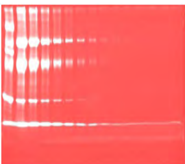
SYPRO Ruby stained SDS-PAGE excited through MD-25 UV transilluminator
