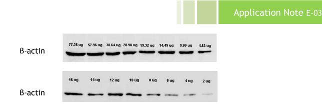
Figure 2. Detection of B-actin within series diluted 293T cell lysate after transfer from 12% SDS-PAGE to PVDF membrane with 25 V for 7 minutes. The number represent in the picture were the amount of total protein in 293T cell lysate that were loaded.
