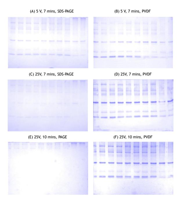
Figure 1. Transfer efficiency of ProMarker Plus with different conditions. Apply with 5V (A) (B) and 25 V (C)
